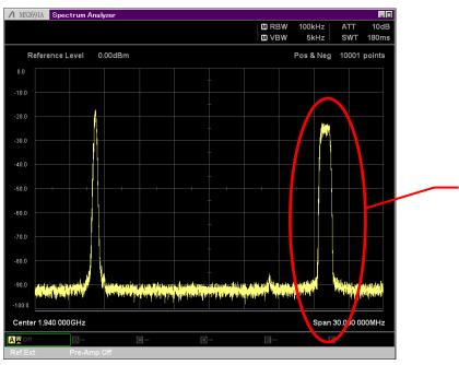
W-CDMA waveform pattern The true bandwidth is about 3.84 MHz but this bandwidth has been changed to output at the combined GSM waveform pattern sampling rate.
