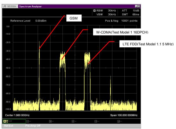
Figure 8. Example of Tx Characteristics Test Signal Output from MG3710A
