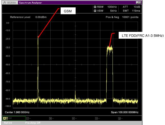
Figure 9. Example of Tx Characteristics Test Signals Output from MG3710A
