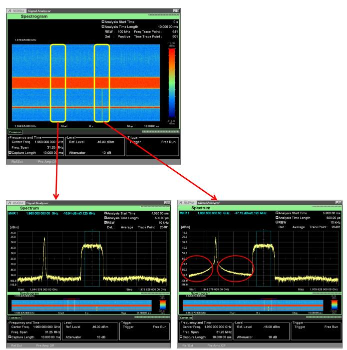
Figure 4. Example of Stopped and Combined Waveform Patterns
