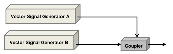
Figure 2. Setup when Combining Outputs from Two Vector Signal Generators
